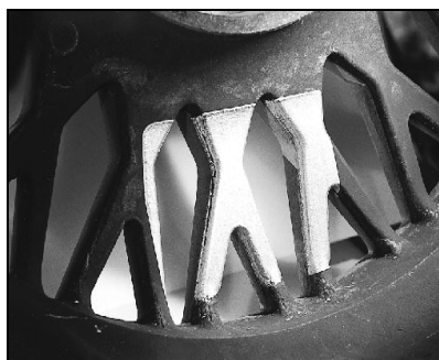
Results of CO2 Blasting
