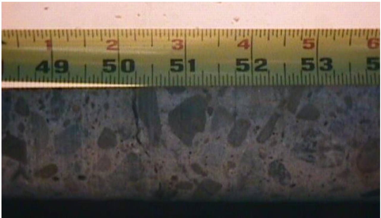
From a 15' core sample...Perpendicular fracture filling at over 50" (1270mm) deep
